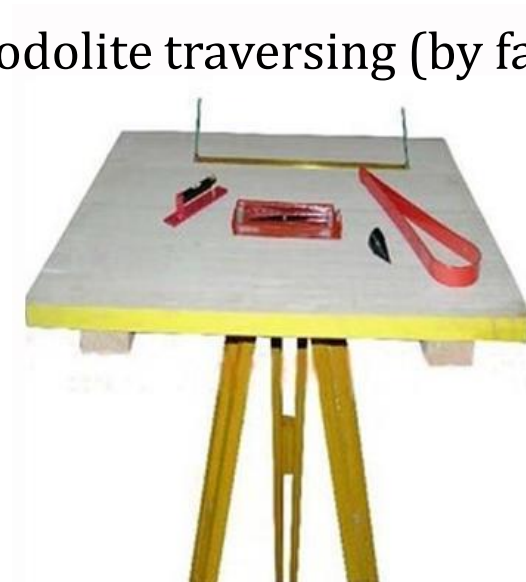
4. Plane table traversing (by plane and table)
