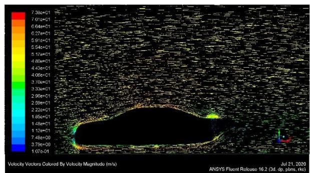
**Fig.11** Velocity vector of the model with 8 vortex generators at  $50 \text{ ms}^{-1}$
