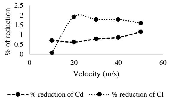
**Fig.14** Reduction percentage of  $C_d$  and  $C_l$  with respect to velocity ( $\text{ms}^{-1}$ )
