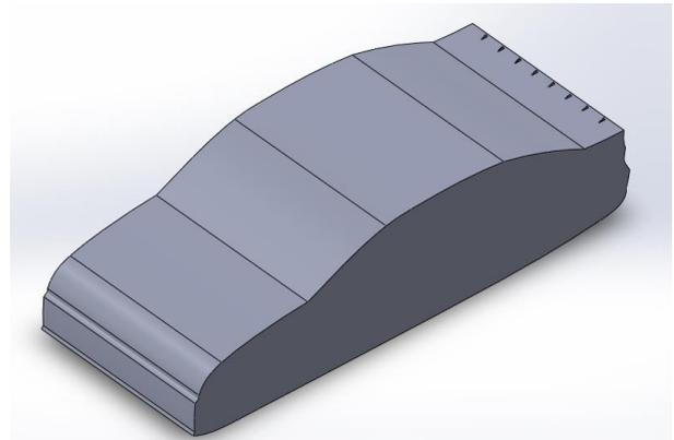
**Fig.3** Car body attached with vortex generators
