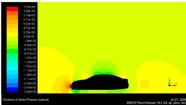
**Fig.8** Static Pressure contour of model without any vortex generator at  $50 \text{ ms}^{-1}$
