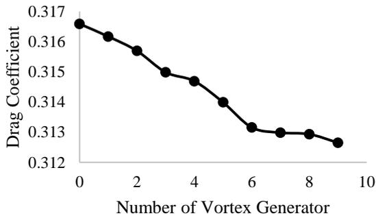
**Fig.7** Plot of  $C_d$  vs number of vortex generators for inlet velocity of  $50 \text{ ms}^{-1}$
