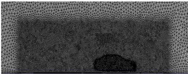
Fig.5 Meshing of the model
