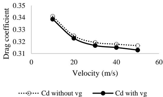
**Fig.12** Comparison of  $C_d$  for both models with respect to velocity ( $\text{ms}^{-1}$ )
