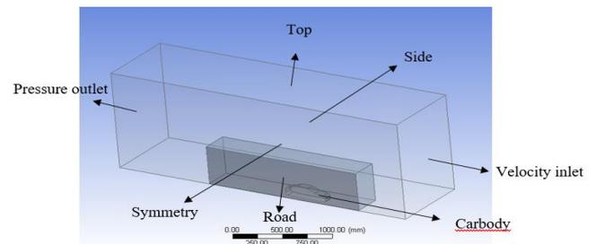
**Fig.4** Enclosure formation in Design Modular
