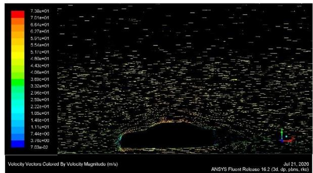
**Fig.10** Velocity vector of the model without vortex generator at  $50 \text{ ms}^{-1}$
