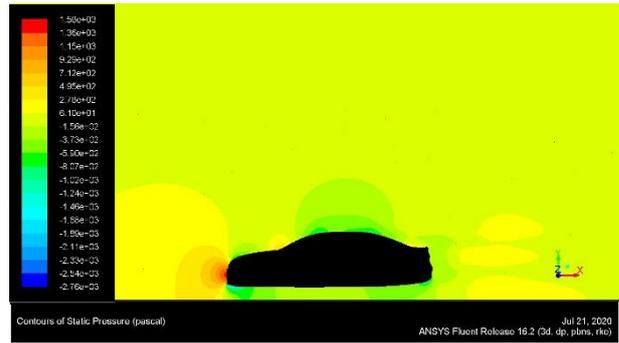
**Fig.9** Static Pressure contour of the model with 8 vortex generators at  $50 \text{ ms}^{-1}$
