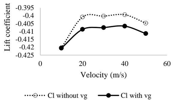
**Fig.13** Comparison of  $C_l$  for both models with respect to velocity ( $\text{ms}^{-1}$ )
