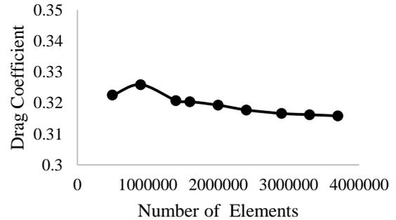
Fig.6 Drag coefficient vs number of elements curve
