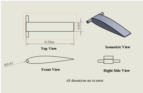
Fig.1 Dimensions of modified NACA 2415 airfoil
