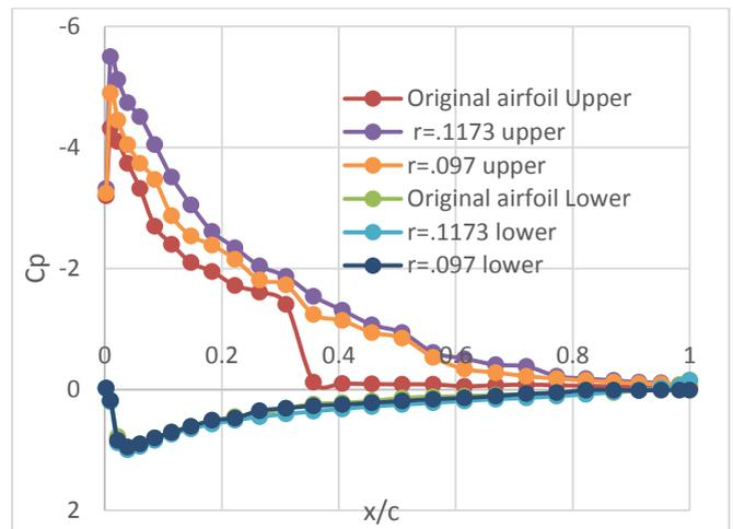
Fig.3 Effect of leading edge rotating cylinder on pressure coefficient,  $C_p$  at 12° AOA.
