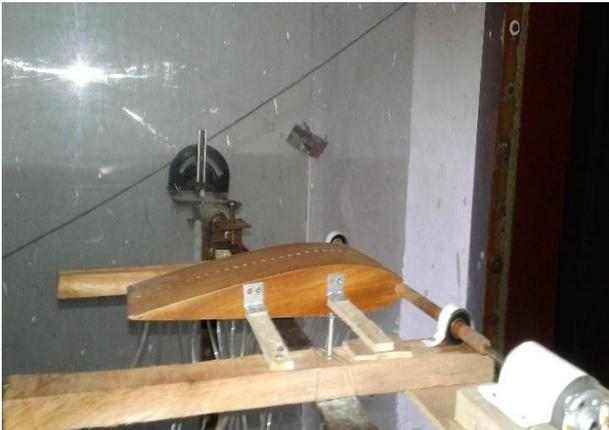
Fig.2 Airfoil mounted on wind tunnel.
