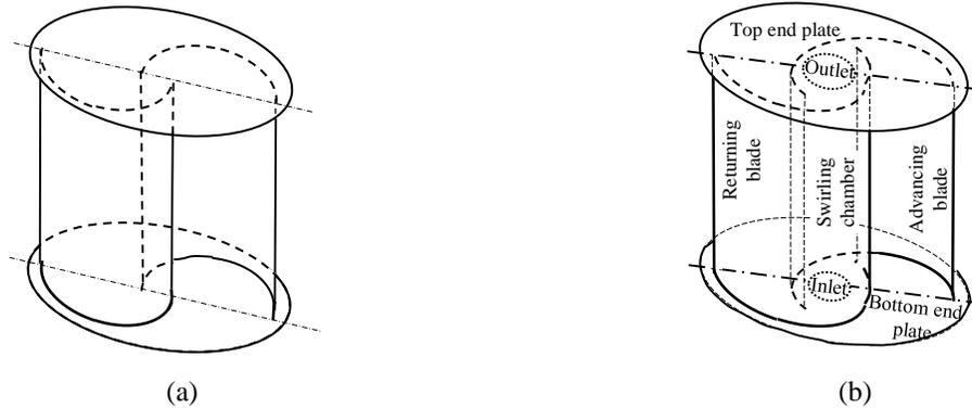
**FIGURE 1.** Schematic diagrams of (a) conventional and (b) Swirling Savonius turbines
