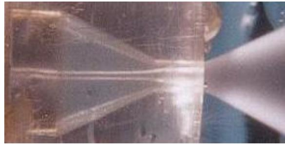
$D_o/D_s = 0.25$ ,  $D_p/D_s = 0.315$ ,  $L_o/D_s = 0.5$ ,  $\alpha = 40^\circ$ ,  $Re = 1.65 \times 10^4$
