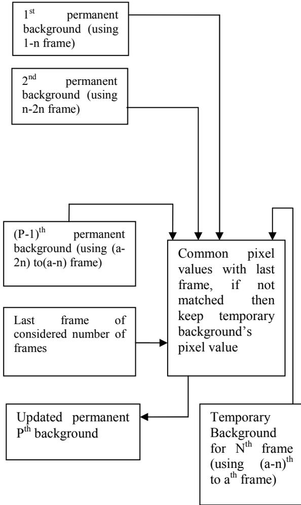
Figure 1. Block diagram for background modeling
