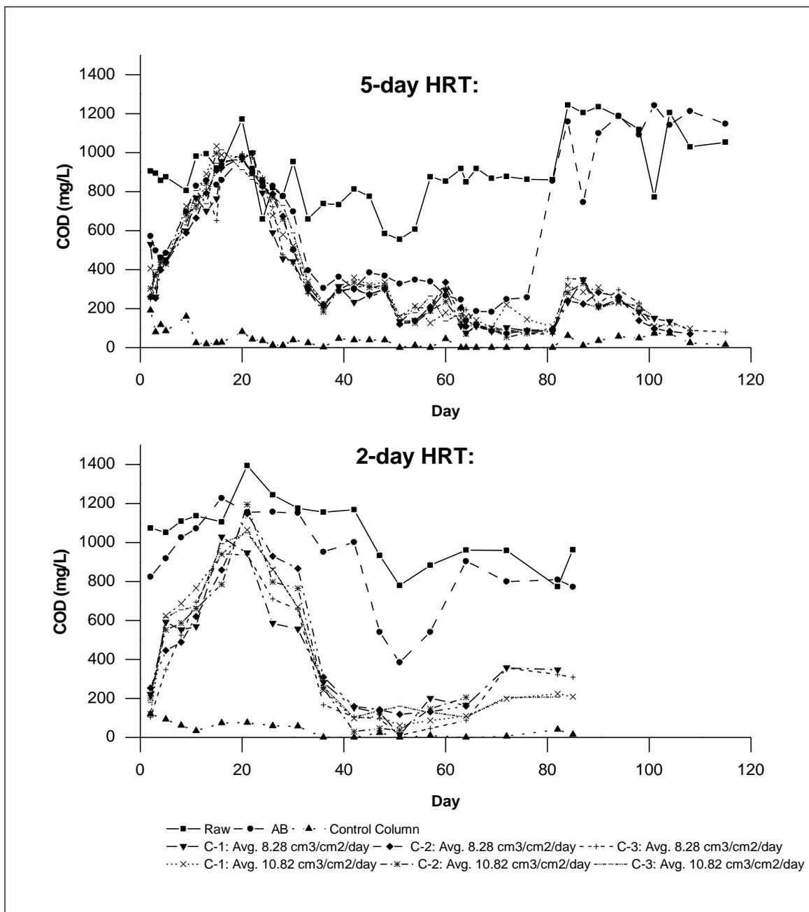
Figure 2 : COD of Raw Leachate, Aerated Leachate, and Column Effluents for the 5-day and 2-day HRTs
