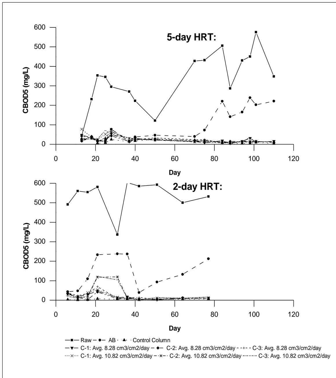
Figure 3 : cBOD<sub>5</sub> of Raw Leachate, Aerated Leachate, and Column Effluents for the 5-day and 2-day HRTs
