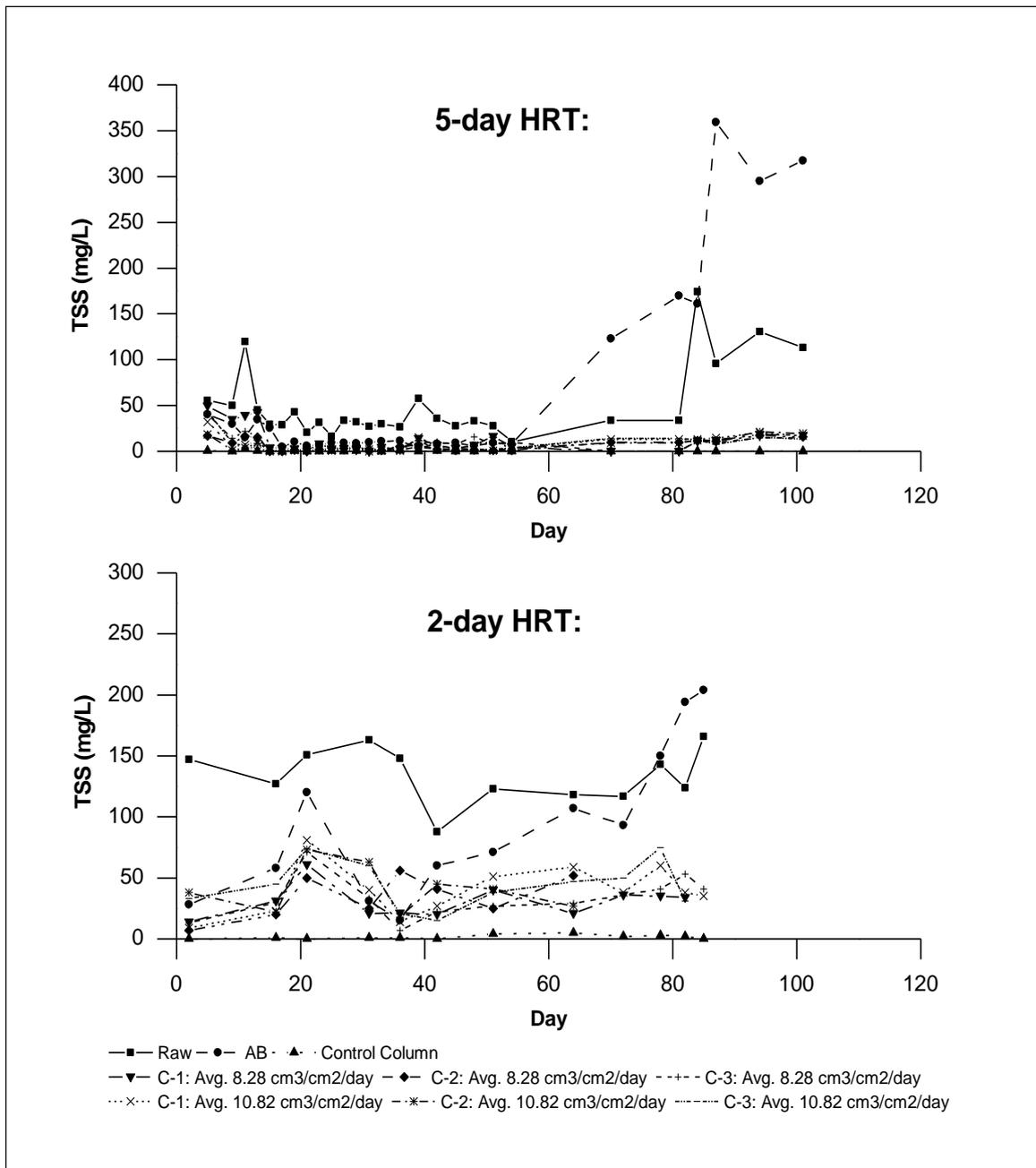
Figure 5 : TSS of Raw Leachate, Aerated Leachate, and Column Effluents for the 5-day and 2-day HRTs
