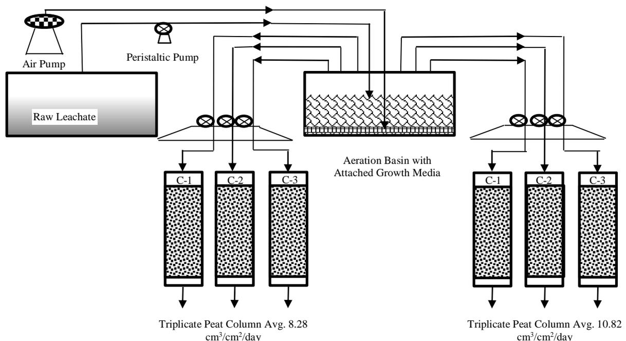
Figure 1 : Sequential aerated peat biofilter experimental set-up under varied loading rates.
