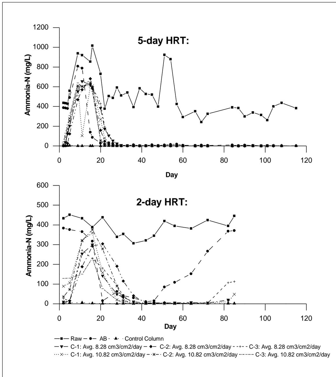
Figure 4 : Ammonia-N of Raw leachate, Aerated leachate, and Column Effluents for the 5-day and 2-day HRTs.
