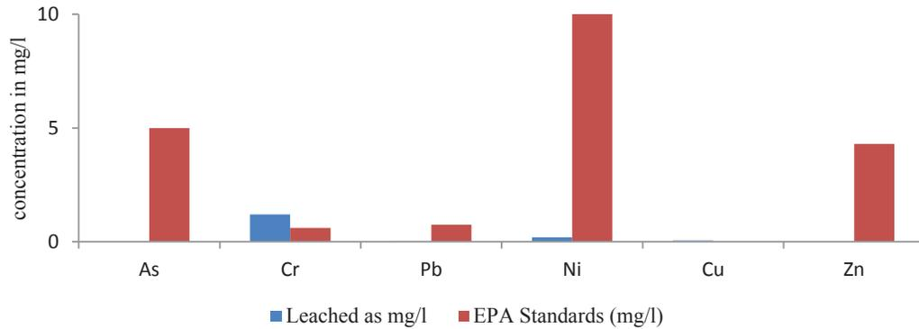
**FIGURE 1.** Results of average concentrations of As, Cr, Pb, Ni, Cu and Zn in Standard TCLP leaching test of leachates from raw sludge and their EPA Standards
