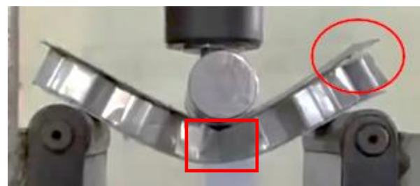
(b) Debonding on one side (circle) and core buckling (rectangle)
