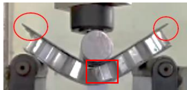
(c) Debonding on both side (circle) and core buckling (rectangle)
