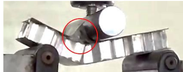
(a) Local debonding
