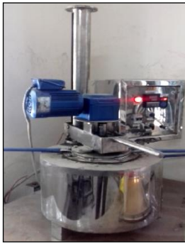
Figure 4: Melting and blending unit.
