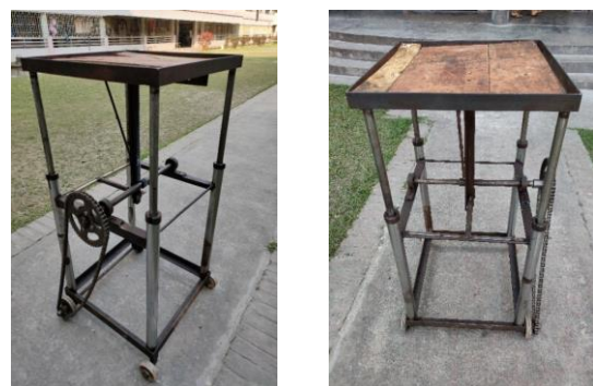
Fig.2 Constructed material handling system (two different views)
