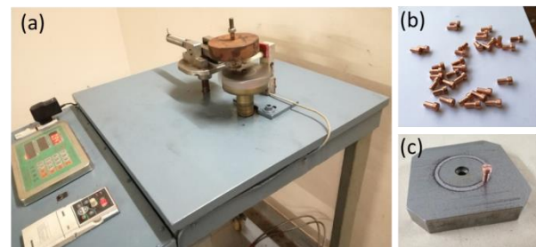
Fig. 1 Experimental setup: (a) Pin-on-disk apparatus, (b) Samples and (c) One sample on the disk.
