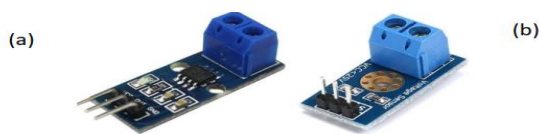
Fig.6 (a) Current Sensor (b) Voltage Sensor
