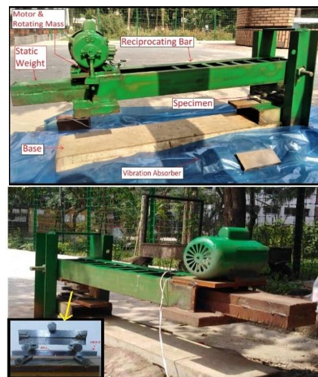
Fig.8 Machine after Complete Fabrication
