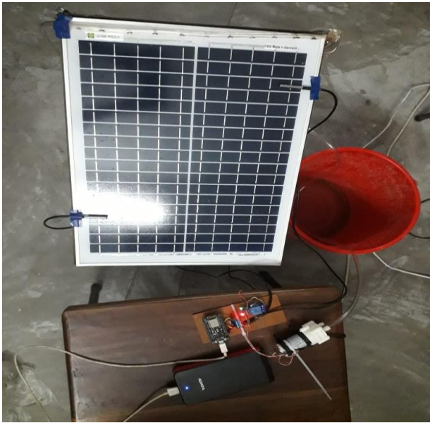
Fig.4 Experimental Setup of components connected with PV module.
