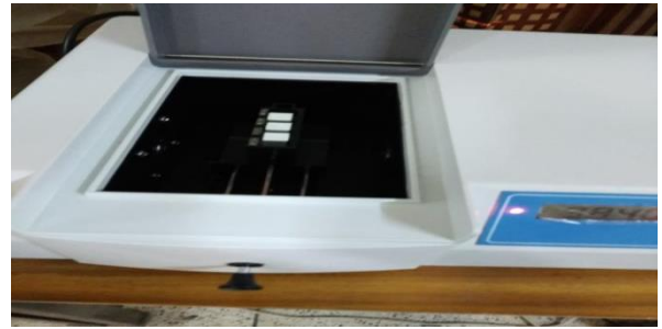
Fig.7 Formaldehyde Release (AATCC Test Procedure 112) Test
