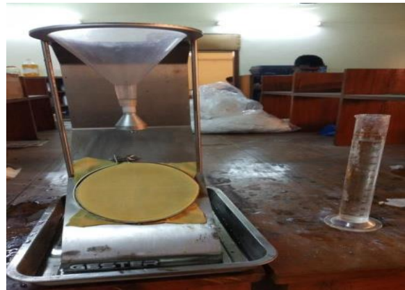
Fig.5 Spray rating test
