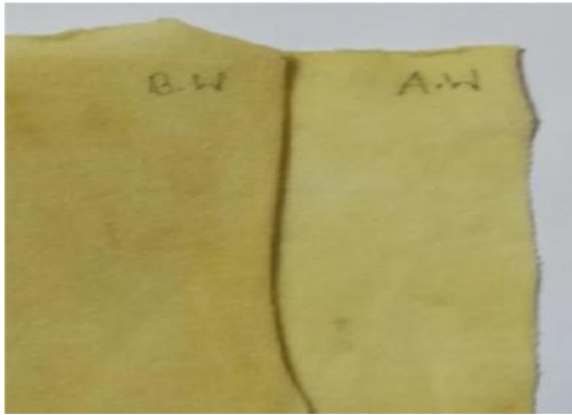
Viscose fabric sample before wash (B.W.) & after wash (A.W.)
