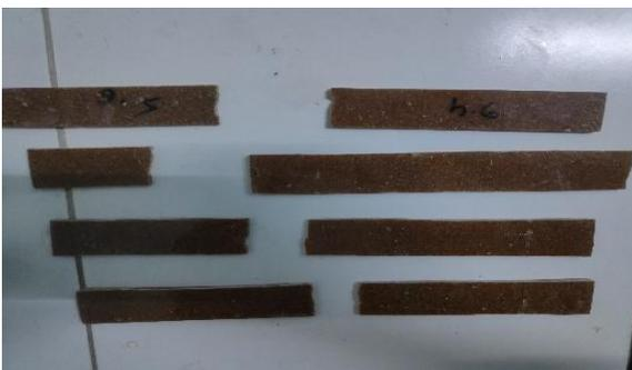
**Fig.5** Specimens After Tensile Test
