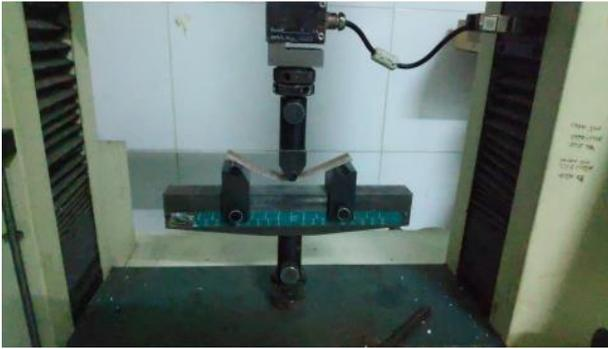
**Fig 2:** Flexural Test Setup
