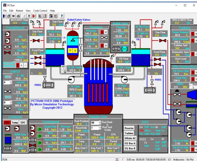
Fig.2 Initiation of 507 cm<sup>2</sup> hot leg LOCA with SBO
