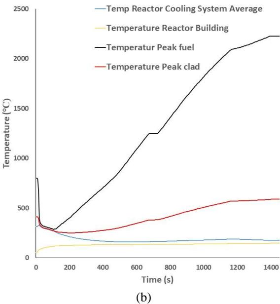
**Fig.6** (a) Pressurizer, SG-A, SG-B, reactor core, reactor building **water level** (m) (b) Peak fuel, RCS average, peak clad, RB **temperature** (°C) (c) Departure from nuclear boiling ratio (d) **Reactivity** of soluble boron, modifier temperature, fuel doppler, rod and total (%) due to LOCA without ECCS at SBO condition
