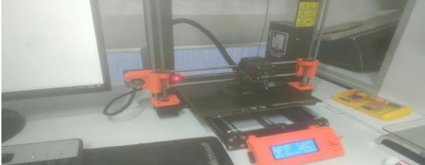
Fig.4 Printing of Spur gear in a Prusa I3 Mk3
