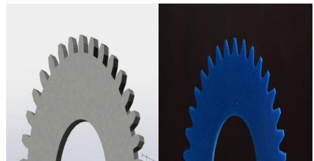
(a)Designed model of Gear (b)Fabricated Gear by Milling
