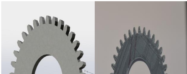
(a)Designed model of Gear (b)Fabricated Gear by FDM
