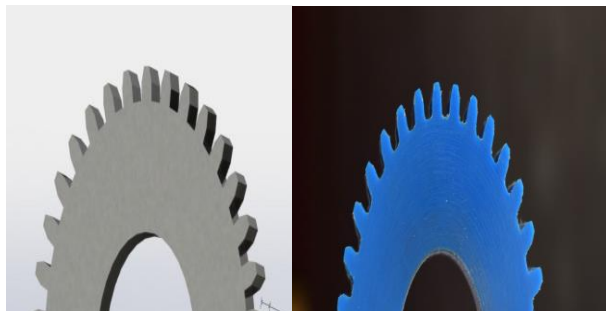
(a)Designed model of Gear (b)Fabricated Gear by CNC Milling
