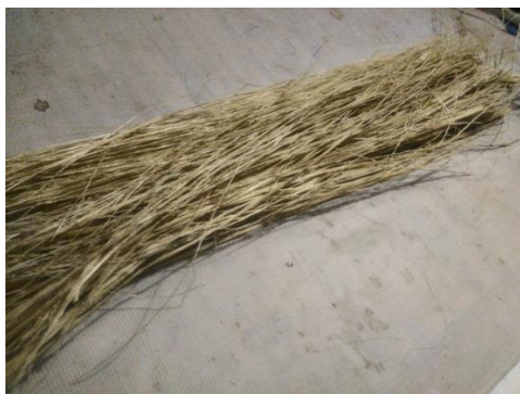
Figure.3 Extracted bagasse fiber
