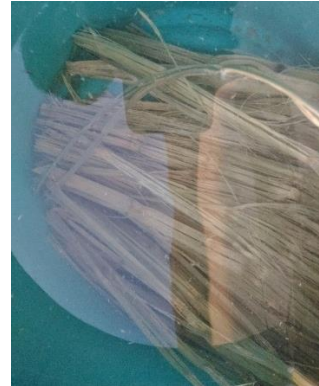
Figure.4 Alkali treatment of Bagasse fiber
