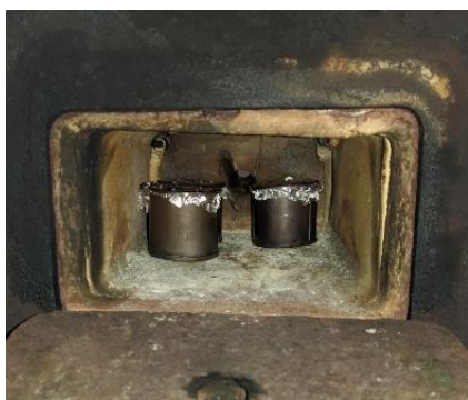
Fig.3 Steel jar placement in muffle furnace
