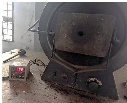
Fig.4 Heating controlled by thermocouple & controller
