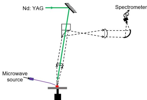
**Figure 1.** MW-LIBS experimental setup
