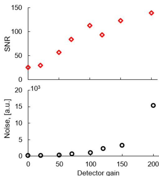
**Figure 2.** Effect of detector gain on signal to noise ratio using CaF molecular emission at 10 mJ laser energy, 600 W microwave power, 400 ns gate-delay, 300  $\mu\text{s}$  gate-width with 100 accumulation.
