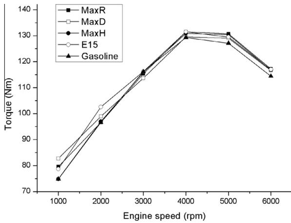
Fig. 3. Variation of Torque with engine speed.
