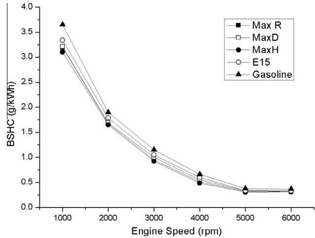
Fig. 8. Variation of BSHC emission with engine speed.
