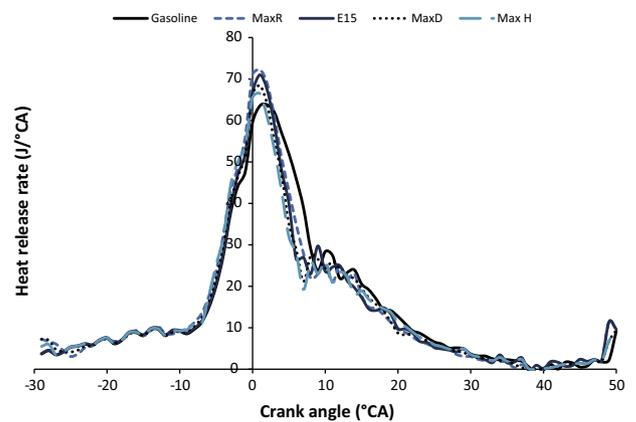
Fig. 6. Comparison of heat release rate at 5000 rpm.
