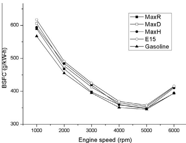
Fig. 4. Variation of BSFC with engine speed.
