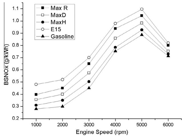
Fig. 9. Variation of BSNOx emission with engine speed.
