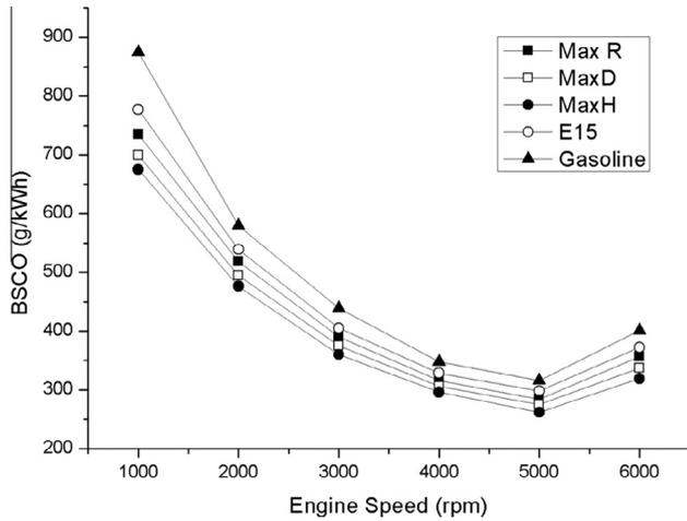
Fig. 7. Variation of BSCO emission with engine speed.
