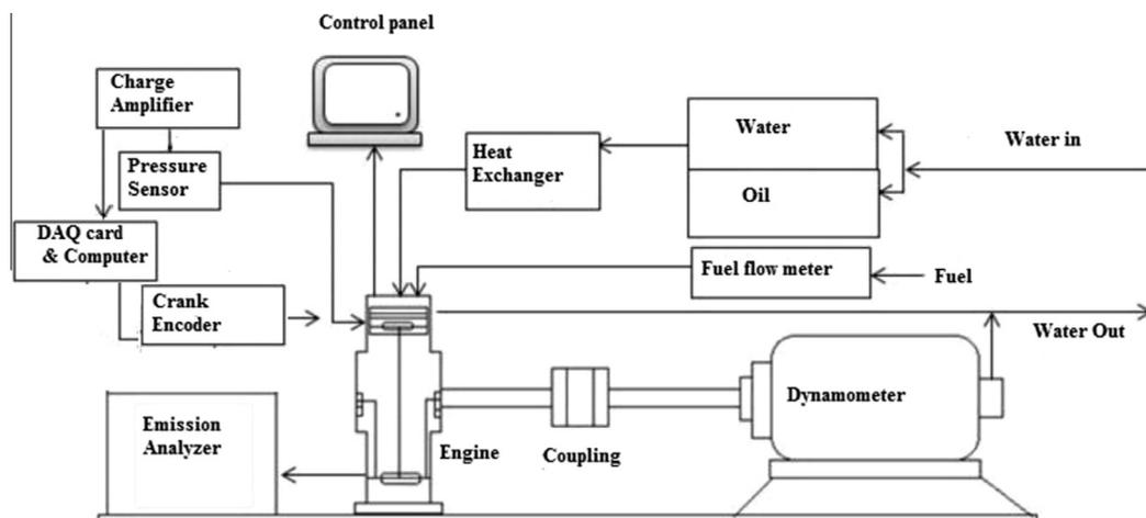
**Fig. 2.** Schematic diagram of the engine test bed.
