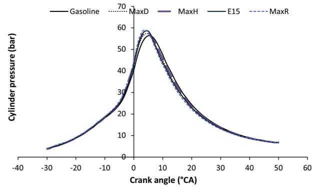
Fig. 5. Comparison of in-cylinder pressure at 5000 rpm.
